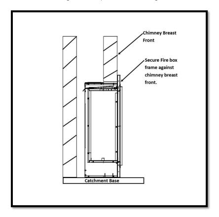
Please note. The P5 fire box assembly must be supported on a flat surface, failure to provide this WILL result in an outing issue on the appliance.
