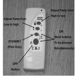
B. The appliance can be adjusted up or down by pressing the h
