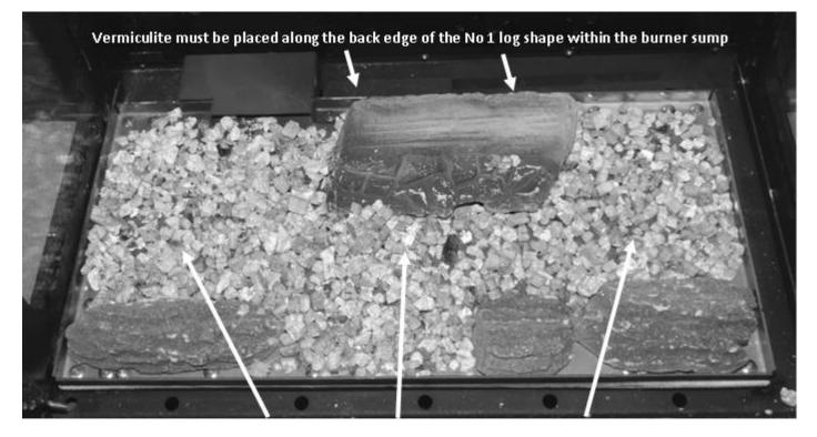
Place a even amount of vermiculite across the complete area of the burner sump.
