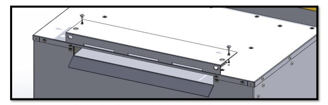
With the plate removed and if spillage is detected the cause must be discovered and the fault corrected. If the fault cannot be corrected, disconnect the fire from the gas supply and seek expert advice. Spillage can be caused by a restriction in the flue, down draught, or insufficient ventilation into the room where the fire is installed.
