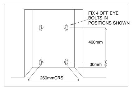
Fix the fire casing back into the opening using the cable fixing system as shown in do not cut off loose ends of cable after fixing, coil and tuck carefully behind sides of Refractory back
