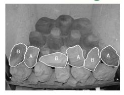
Add the second row of 3 x A and 2 x B loose coals on to the matrix, resting against the previously placed row of coals and the base matrix. DO NOT allow the coals to fall down the gaps between the matrix peaks.
