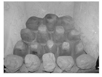
Place the first row of 3 x A and 3 x B overlay loose coals as shown between the front coals and base matrix. Make sure that they are stable and DO NOT let them fall down in the gaps between the peaks on the matrix.
