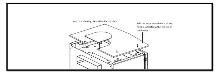
Note:- When installing the appliance using the above method. The appliance must sit hard against the closure place. This will allow 50mm of the rear spigot assembly to protrude into the catchment area.
