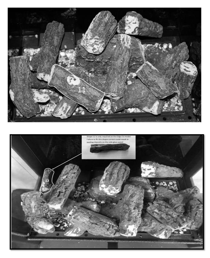
Please note the number 12 shape is only included with the Edge 3s fuel bed. Failure to fit this shape correct could result in sooting deposits on the side glass window. The shape should be place directly on the burner tray alongside the pilot shield.
