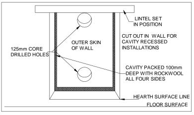
Pass a tape measure through the core-drilled holes and record the distance from the back of the spigots to the surface of the outside wall.
