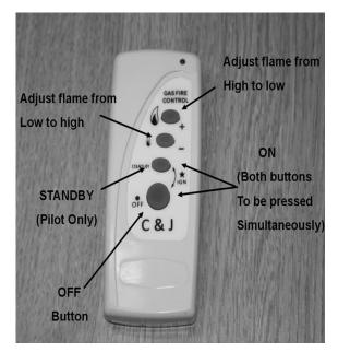
will automatically go to the high setting (approximately 20-25sec). If the ignitor stops sparking and the pilot fails to light, repeat this procedure.
