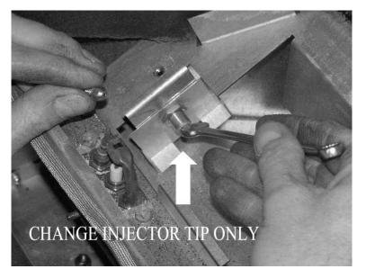
Refit the burner bar by sliding the left hand side first, make sure not to damage the injector tip when replacing burner bar.
