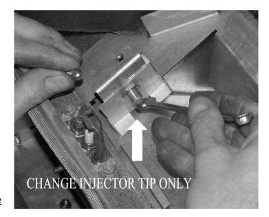
Refit the burner bar by sliding the left hand side first, make sure not to damage the injector tip when replacing burner bar.
