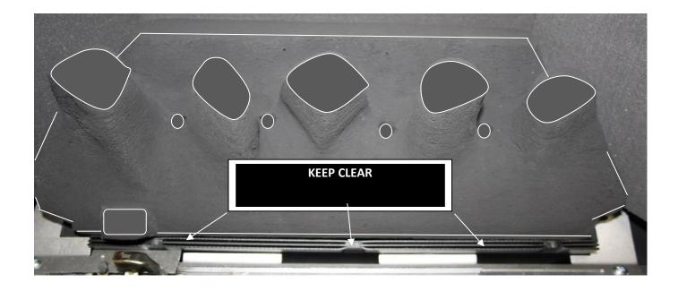
• When positioning the rear matrix be careful not to cover the burner ports
