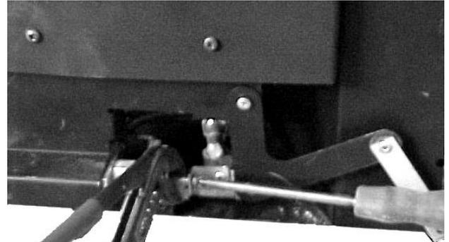
Check for gas soundness. Reconnect the bell crank mechanism as above ensuring that the gas control spindle is gripped only over the protective copper sleeve and no other part of the spindle as, ensure NO side strain is applied to the spindle.
