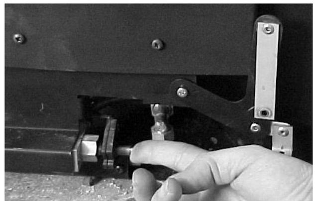
Ensure the spindle is pushed back inside the control valve as far as possible. Ensure the bell crank mechanism is swung up to give easy access to the gas connection point as shown.
