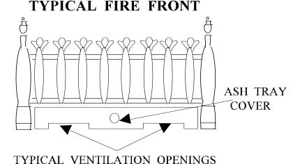
• The ash tray cover must have cut-outs and or holes which provide ventilation to the underside of the burner. The effective area of ventilation through the ash tray cover must be greater than 1365mm2 (2.12 sq. ins.).
