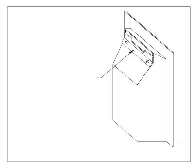
**Note:** A brick or stone chimney with a 125 mm (5 ins) minimum diameter flue liner conforming to BS 715 may be used. Provided a suitable sealing plate is fitted to the base of the liner and the appliance does not restrict the opening into the liner.
