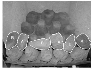
Add the second row of 3 x A and 2 x B loose coals on to the matrix, resting against the previously placed row of coals and the base matrix. DO NOT allow the coals to fall down the gaps between the matrix peaks.
