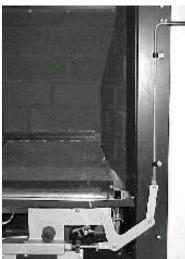
Connect the link lever to the stud at the end of the slide control lever and replace the nylock nut.
