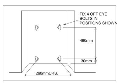
Fix the fire casing back into the opening using the cable fixing system as shown in do not cut off loose ends of cable after fixing, coil and tuck carefully back
