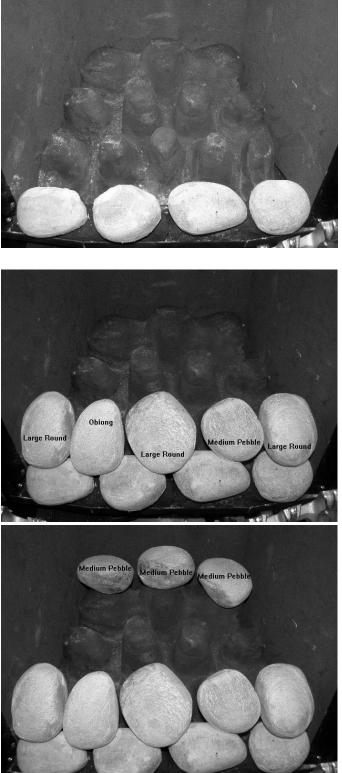
Place two heart shaped pebbles as shown on the second row of pebbles. Rest them carefully on the side liners and base matrix touching the first row laid earlier.
