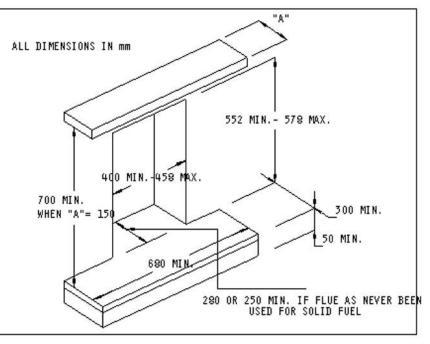
must be added to the minimum 300mm hearth depth to comply with regulations.
