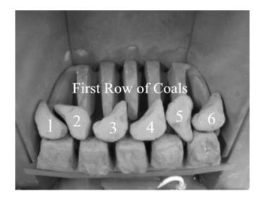
Place the second row of five coals as shown. Ensure the coals bridge across the existing coals and the rear matrix and are stable. Press each one with your fingers to be sure that they are stable and will not fall through on to the burner. Re-position carefully as required.
