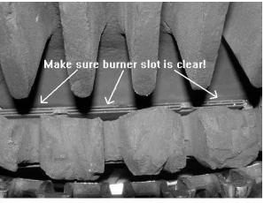
slide front coal support on to the edge of the burner carrier this will support the front coal matrix and help stabilize the fuel bed
