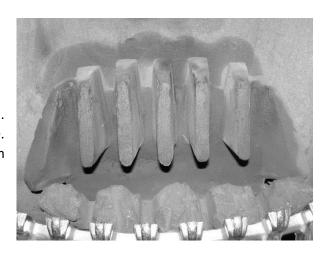
Locate the front coal matrix with the shapes upwards in front of the rear matrix. Ensure that it is not placed on top of the burner slot.
