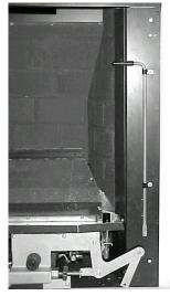
Flip the slide control lever round so that the rubber-capped end is protruding out to the right as shown in the left-hand picture. Check that it slides freely up and down in the nylon slide guides. Remove the nylock nut with a 7mm A/F spanner as shown.
