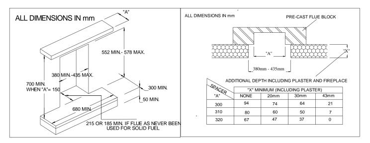
NOTE:- LOW LINTEL OPENING HEIGHT IS REDUCED TO 500mm - 526mm.
