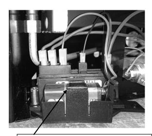
Ensure battery is located properly so this hook hold the battery in place
