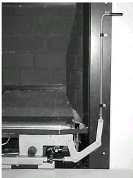
the end of the slide control lever and replace the nylock nut.
