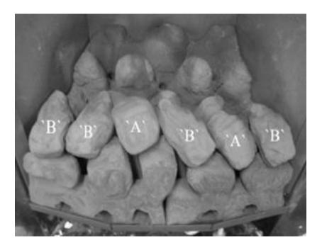
Lay second row of loose coals 3 off "B" and 2 off "A" shapes as shown.
