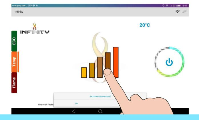
Press and hold the **Temperature Bar Chart** area of the screen until a **Set current temperature** message screen appears.
