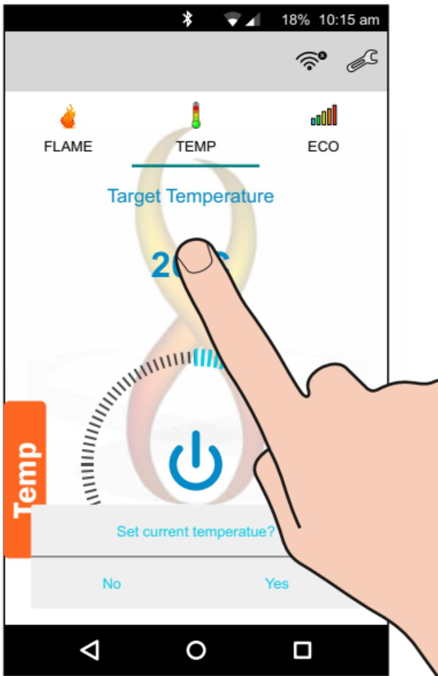
Press and hold the **Target Temperature** area of the screen until a **Calibrating to** message screen appears.
