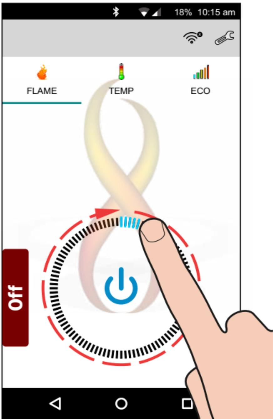
Secondly drag the heat dial clockwise from minimum to maximum.
