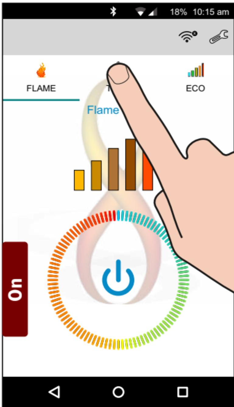
To calibrate the thermostat tap the **Temp** mode icon
