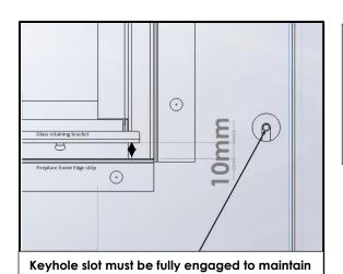
the 10mm clearance between the glass fixing bracket and the bottom internal edge of the
