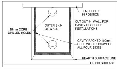
Pass a tape measure through the core-drilled holes and record the distance from the back of the spigots to the surface of the outside wall.
