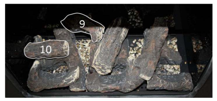
Place log 9 on the peg from log 8 so it bridges the gap. Place log 10 on its location peg as shown.
