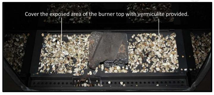
Place a <u>VERY</u> thin layer of vermiculite over the burner as shown.
