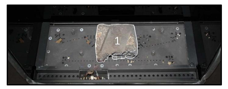
Place shape No1 directly onto the studs as shown.
