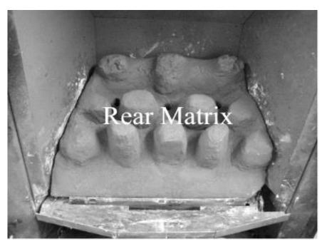
Locate the LEFT HAND and RIGHT HAND FRONT COALS as shown so that they sit on the front rail and lean back against the BASE MATRIX. Note it is most important that they are located in their correct positions. They are marked on the rear "L" for LEFT HAND FRONT COAL and "R" for RIGHT HAND FRONT COAL.
