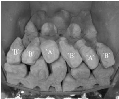
Lay second row of loose coals 3 off "B" and 2 off "A" shapes as shown.
