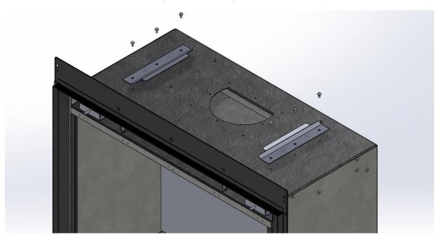
Offer the fire box assembly within the masonry aperture at the same time guiding the Outlet Assembly within the guides situated on the top of the fire box (Please see Fig 2). Slide the Outlet Assembly towards the front flange and secure using the three Self Tapping screws provided within the Outlet Assembly kit.
