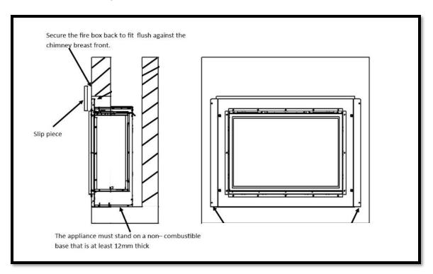
Using rawl plugs and wood screws retain the fire box via the holes in the Fireplace Frame. None combustible slips can now be fitted up to the edge of the fire place frame.
