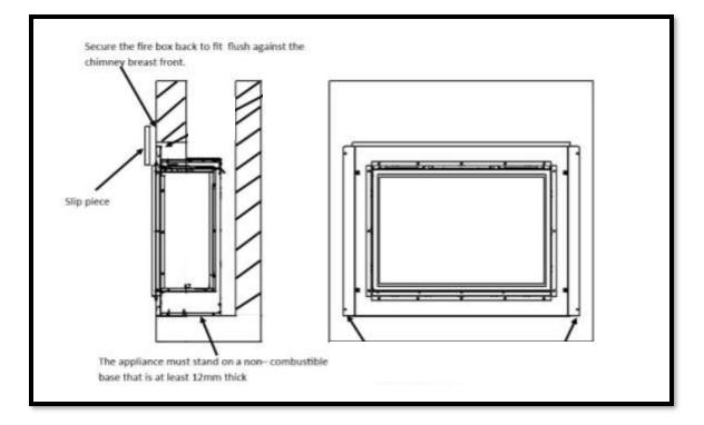
Using rawl plugs and wood screws retain the fire box via the holes in the Fireplace Frame. None combustible slips can now be fitted up to the edge of the fire place frame.
