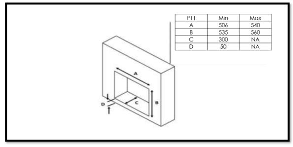
A-B-C / Builder's opening aperture size when fitting hole in the wall boarded edge or slips.
