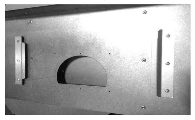
Offer the fire box assembly within the masonry aperture at the same time guiding the Outlet Assembly within the guides situated on the top of the fire box (Please see Fig 2). Slide the Outlet Assembly towards the front flange and secure using the three Self Tapping screws provided within the Outlet Assembly kit.
