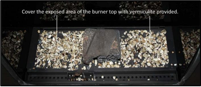
Place a **VERY** thin layer of vermiculite over the burner as shown.
