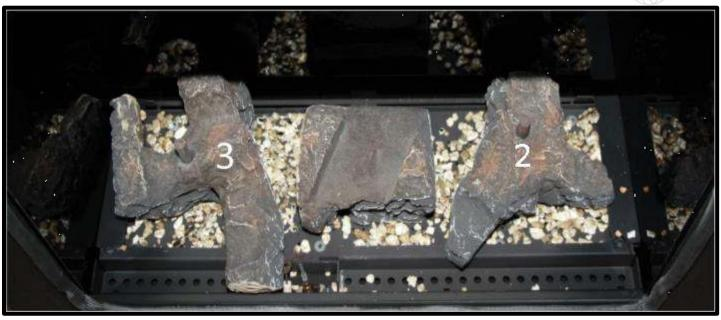
Place Logs No2 & No3 on top of the studs in the positions shown.
