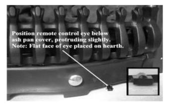
Check that a signal is being received by pointing the remote control hand set in the direction of the appliance and simultaneously press the buttons marked <sup>(•)</sup> and 'standby'. Continue to hold in these two buttons until a 'bleep' is heard (approximately 2-3 sec.). If no sound is hear check position of remote control eye.
