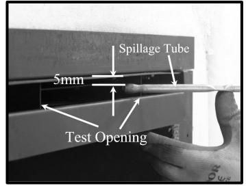
• If spillage is detected the cause must be discovered and the fault corrected, if the fault cannot be corrected, disconnect the fire from the gas supply and seek expert advice. Spillage can be caused by a restriction in the flue system, down draught or insufficient ventilation into the room where the fire is installed.
