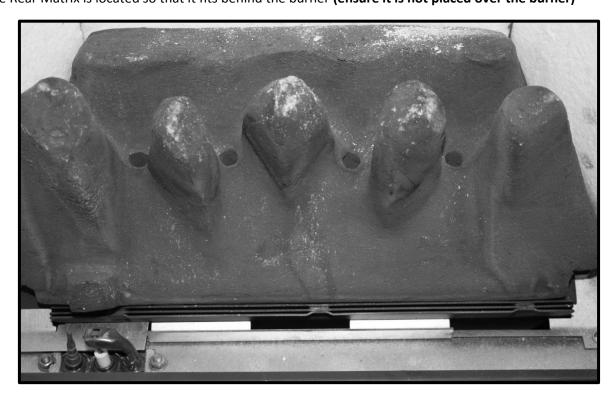
When positioning the rear matrix be careful not to cover the burner ports
