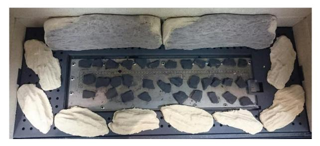
• Place a single layer of black bark chippings across the burner top plate. Place two off the log shapes along the back edge of the air tray as shown. Finally place a single layer of the large bark chippings along the front and sides of the air tray.
