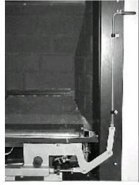
Connect the link lever to the stud at the end of the slide control lever and replace the nylock nut.
