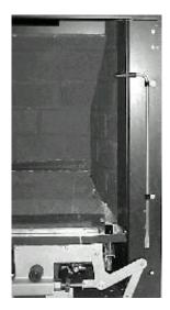
Flip the slide control lever round so that the rubber-capped end is protruding out to the right as shown in the left-hand picture. Check that it slides freely up and down in the nylon slide guides. Remove the nyloc nut with a 7mm A/F spanner as shown.
