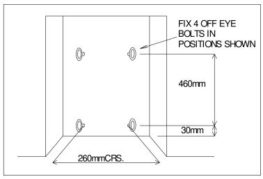
Fix the fire casing back into the opening using the cable fixing system as shown in do not cut off loose ends of cable after fixing, coil and tuck carefully back
