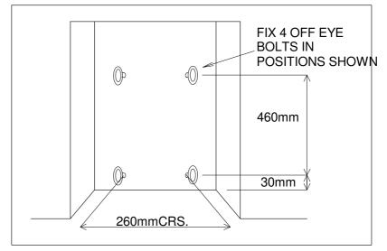
Fix the fire casing back into the opening using the cable fixing system as shown in do not cut off loose ends of cable after fixing, coil and tuck carefully behind burner tray.
