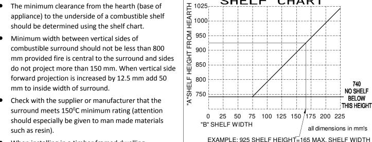
reference must be made to the specific installation requirements stated in Section 10 Installing The Appliance In
