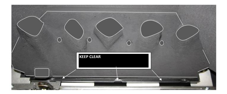
When positioning the rear matrix be careful not to cover the burner ports
