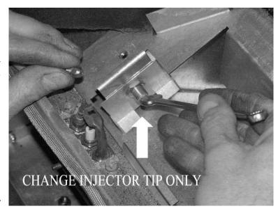
Refit the burner bar by sliding the left hand side first, make sure not to damage the injector tip when replacing burner bar.
