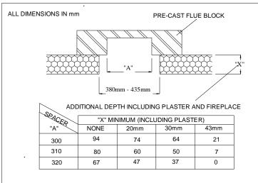
Fireplace opening must be 552 mm - 578 mm high by 380 mm – 435 mm wide (or up to 458 mm if the cable fixing system is used).
