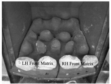
Lay one row of pebbles at the front of the fire as shown. A second row (number positioned against the rear of fire) is placed between the base matrix and the rear of the fire as shown.
