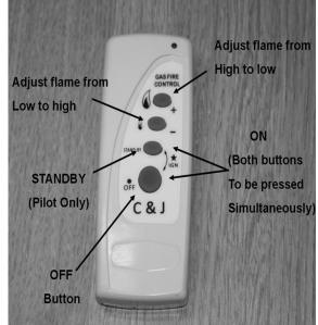
B. The appliance can be adjusted up or down by pressing the appropriate button  $\diamond$  (low setting) or  $\diamond$  (high setting). There are 5 heat settings and the fire will give a double bleep when the maximum or minimum heat
