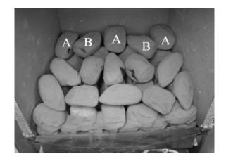
\* Before fitting the pebble set loosen the burner securing screws and make sure that burner is pushed to the right side of the burner tray. This will ensure maximum aeration to the burner and reduce discolouration.
