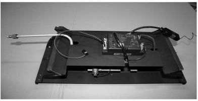
• Connect the Gas Inlet Pipe to the Restrictor Elbow and check for soundness refit Airtrays and commission appliance.
