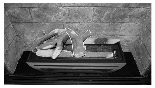
• Place the Thick Middle shape as shown, so it rests on the top of the front R/H shape as shown.
