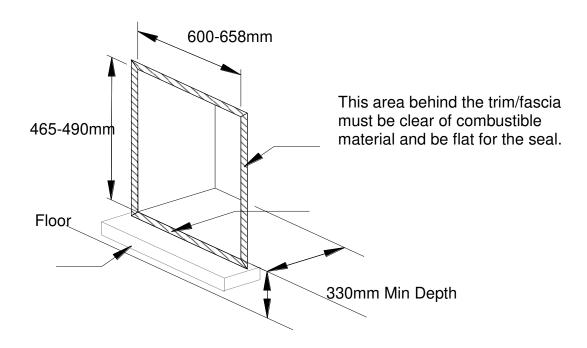
The front face and the base of the fire opening must be flat to ensure that a good seal is formed between the rear and base of the appliance and the chimney to avoid any reduction of natural draught.
