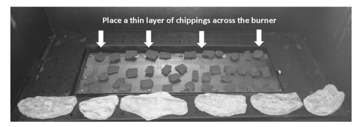
Place air tray within burner shelf assembly and cover the burner plate with a thin layer of chippings. (NG ONLY)
