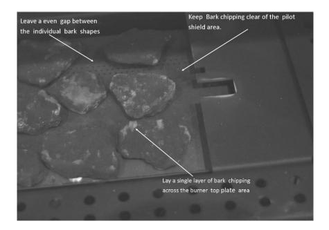
• Please make sure no loose shapes are placed directly on top of the pilot shield. (Please see figure above.
