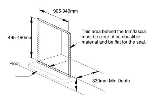
The front face and the base of the fire opening must be flat to ensure that a good seal is formed between the rear and base of the appliance and the chimney to avoid any reduction of natural draught.
