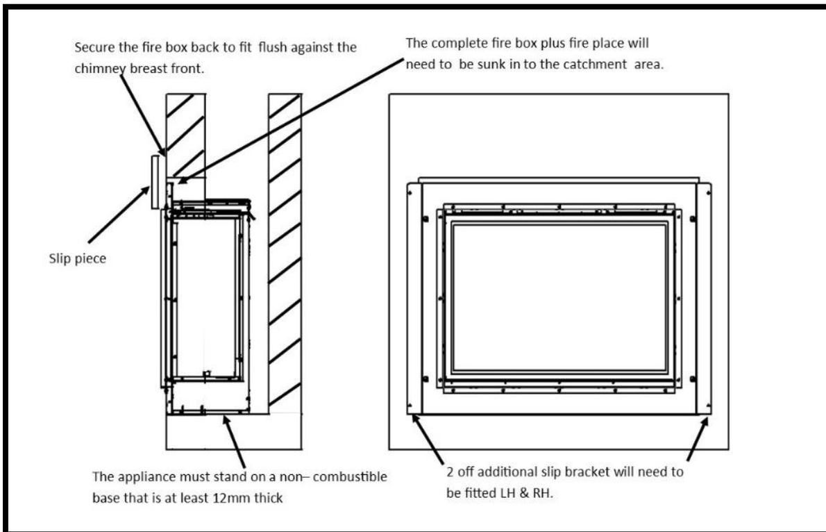
Using rawl plugs and wood screws retain the fire box via the 6mm holes within the slip brackets. None combustible slips can now be fitted up to the edge of the fire place frame.
