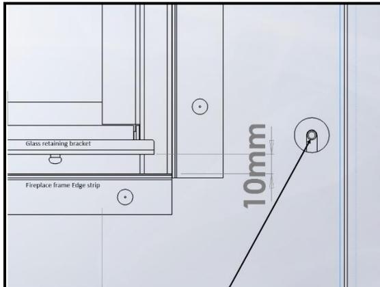
**Keyhole slot must be fully engaged to maintain the 10mm clearance between the glass fixing bracket and the bottom internal edge of the fireplace frame**
