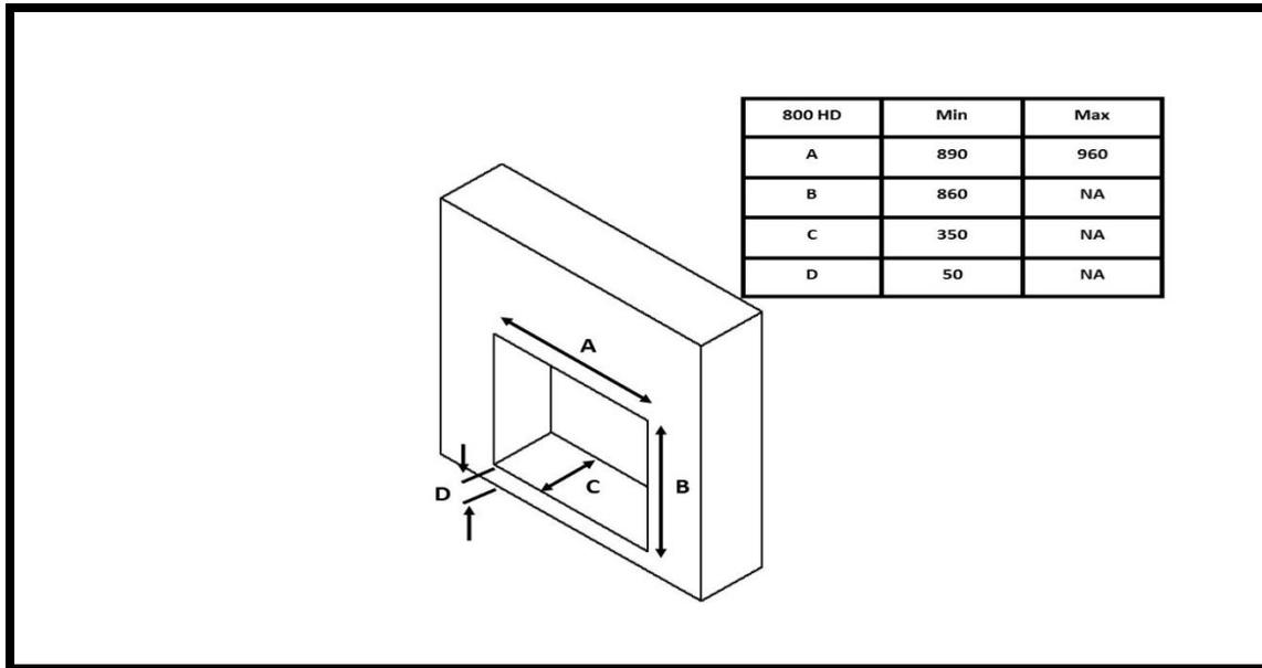
**A-Hole in the wall using none combustible slips.**
