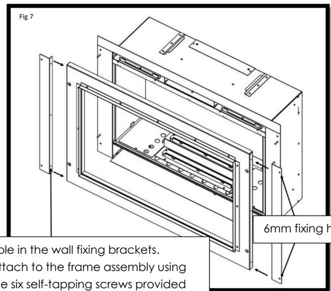
Hole in the wall fixing brackets. Attach to the frame assembly using the six self-tapping screws provided
