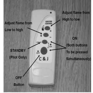
B. The appliance can be adjusted up or down by pressing the  $\mathbf{x}$
