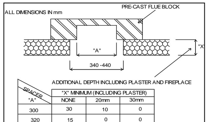
**IMPORTANT: - Do not fit the restrictor plate if the appliance is installed into this type of flue.**
