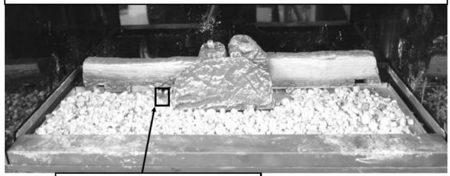
Avoid placing the vermiculite on the cross lighting ports
