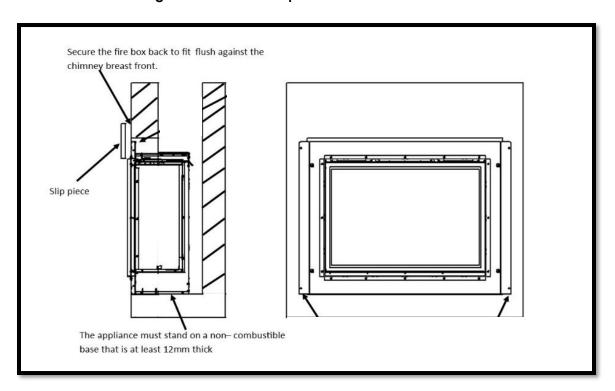
Using rawl plugs and wood screws retain the fire box via the holes in the Fireplace Frame. Noncombustible slips can now be fitted up to the edge of the fireplace frame.
