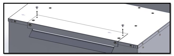
Please fit the 55mm castle cut out restrictor plate provided with the appliance and repeat the spillage test procedure.
