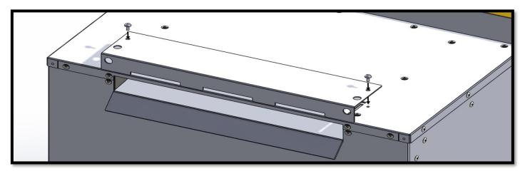
If the appliance continues to give a negative spillage result the 55mm castle cut out should be removed and tested without any restrictor plate fitted.
