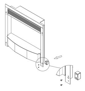
Follow the steps from 5.7a to 5.7e for the detailed installation under the 22' opening dimension.
