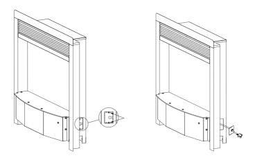
Fix the metal plate with two ST4×10 screws and connect the mood light strip various lengths available
