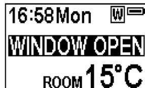
6b.36 After the indoor temperature has risen or a manual override of the warning (by operating remote control) has been done, the fire will return to normal working state.
