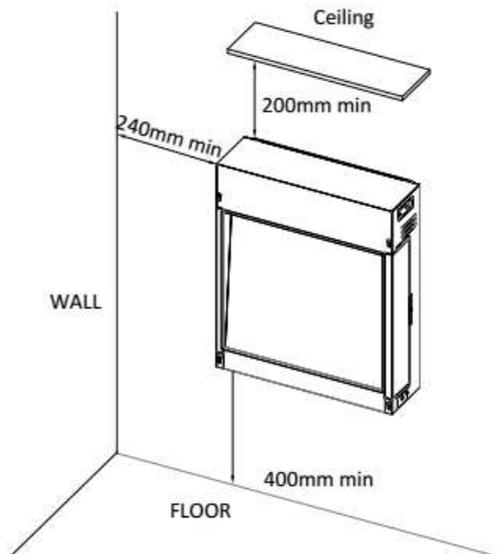
5.5a Carefully, mark and drill four holes on the wall using the wall bracket as a template and push in the four plastic wall anchors. Fix the wall mount bracket onto the wall with four ST5\*40 screws.
