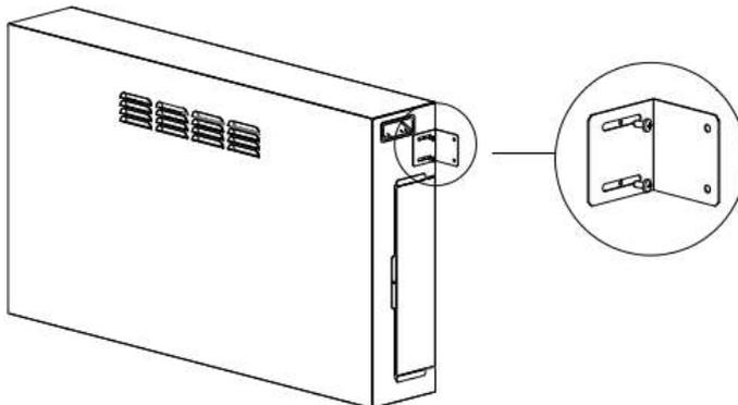
5.4b Push the appliance into the opening hole and then fix the brackets to the wall framework from the front or rear to suit with four ST4\*12 screws.
