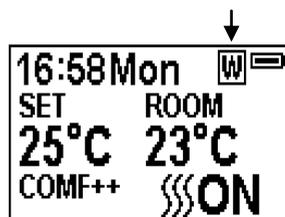
6b.27 Press **M** until **W** shows at the upper right corner of the screen, then enter the week timer heating mode.
