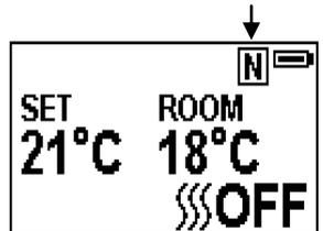
6b.15 Press **⏏ A** button to turn on/off heat, **⏏ON**、**⏏OFF** will show at the lower of the screen.
