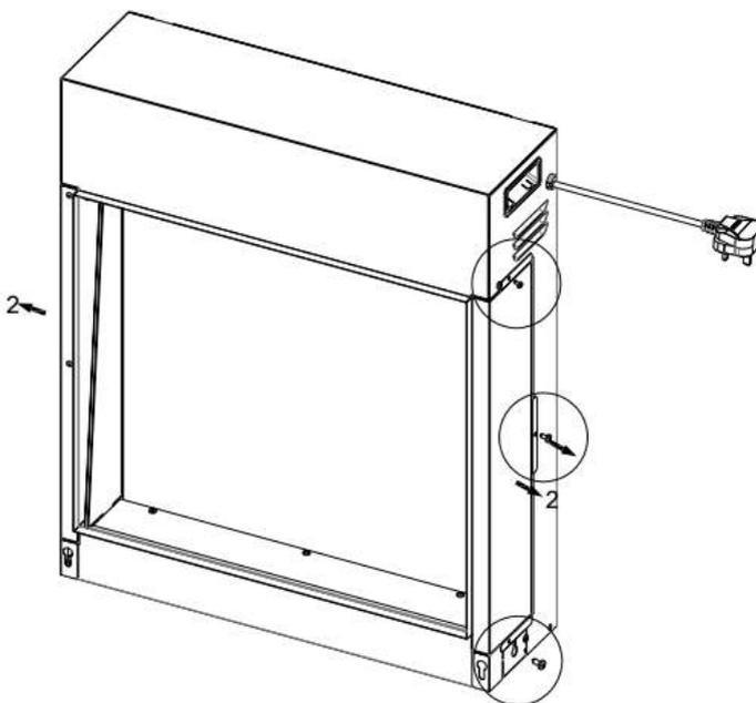
5.5c Put the fire box onto the wall bracket and then fix with two fixing screws of the wall mount brackets on the top of the fire box. Remove the front glass and arrange the fuel bed as described in 5.4c and 5.4d.
