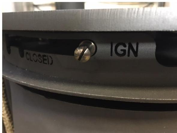
inwards and downwards into the slot until it latches fully into the **CLOSED** position allows the baffle flap to remain in the closed position permanently during all operation. This is useful where flue draw is very good even when the flue is cold.
