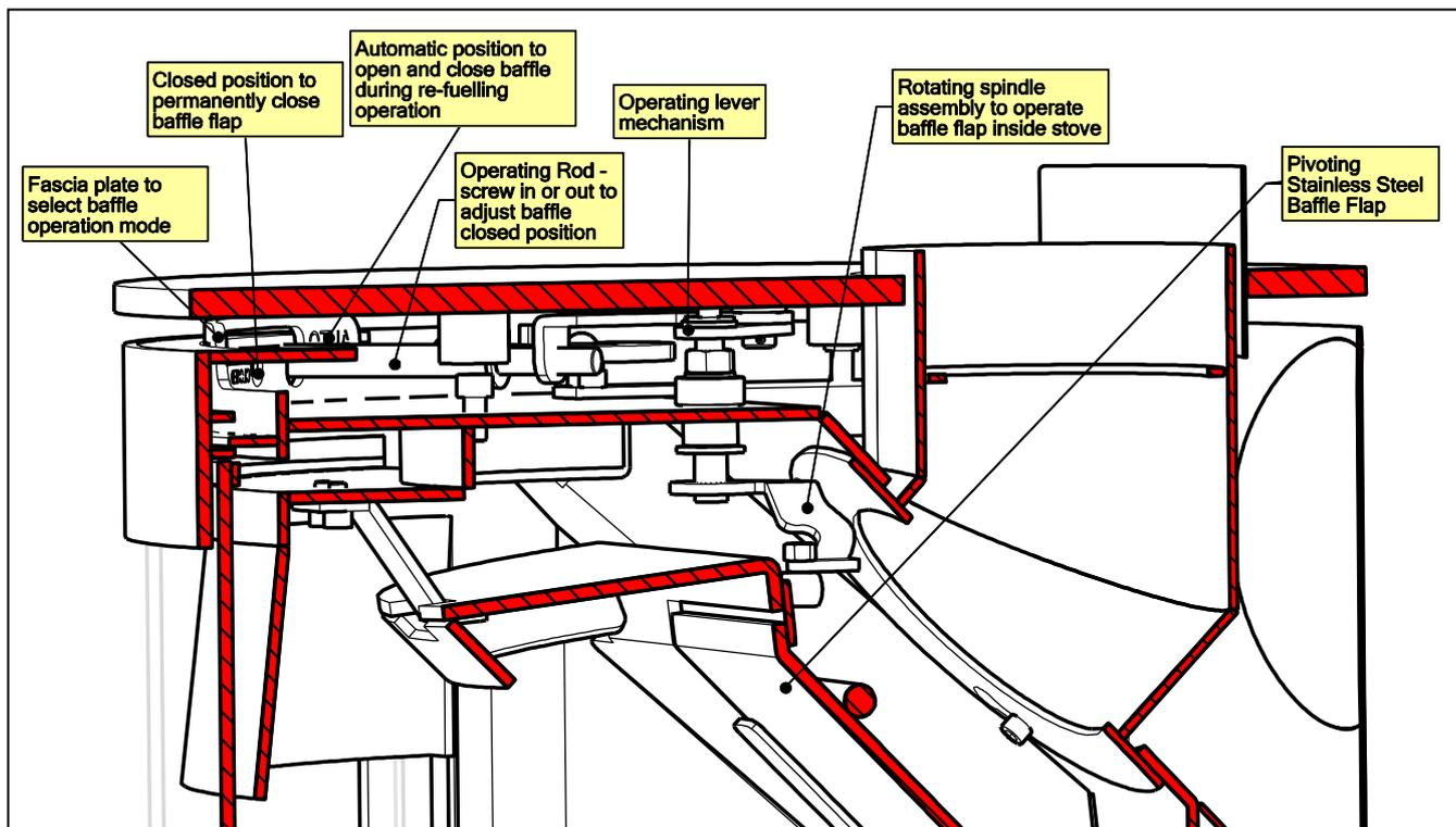
**7.1 Description:** The Purevision PVR range may be fitted with an internal stainless steel active baffle assembly which fulfils a number of functions:
