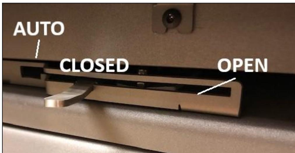
1. **AUTO:** Used when the stove is in normal operation, the baffle will open with the door to reduce any fume emission into the room when re-fuelling and return to the closed running position when the door is closed.
