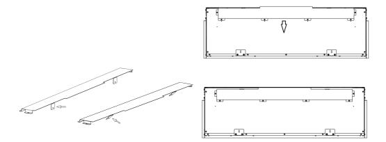
5.7b2 Measure from the lowest point of the appliance to the top edge of the wall bracket. Note: - the wall bracket is currently fixed to the rear of the appliance.
