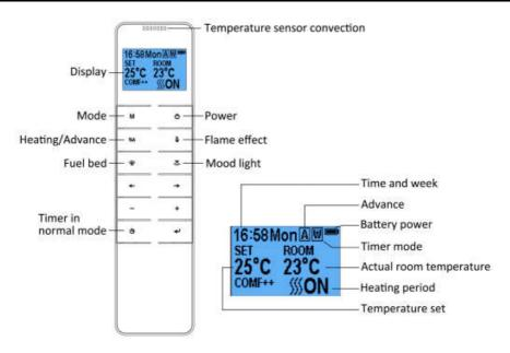
NOTE: This is thermostatic remote control. The remote should be in the same room as fireplace and placed on a flat surface. It must be placed away from the fire so the hot air will not blow on it and affect thermostatic reading.
