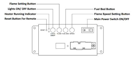
NOTE: The manual button controls basic functions, not a full range of controls. Use the remote hand set to carry out all functions.
