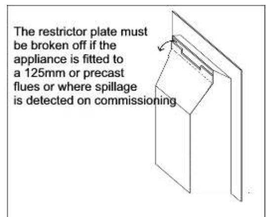
**IMPORTANT: - the flue restrictor plate must be removed when the appliance is installed in this type of flue.**
