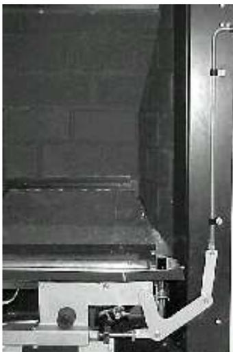
Connect the link lever to the stud at the end of the slide control lever and replace the nylock nut. **IMPORTANT TURN THE NUT UNTIL IT JUST TIGHTENS AND THEN TURN IT BACK A HALF TURN.** Check the operation on the lever and mechanism ensure that the lever springs back to the low position when it is released after pushing down.
