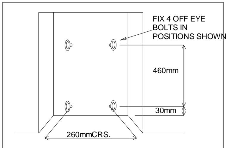
Fix the fire casing back into the opening using the cable fixing system as shown in do not cut off loose ends of cable after fixing, coil and tuck carefully back
