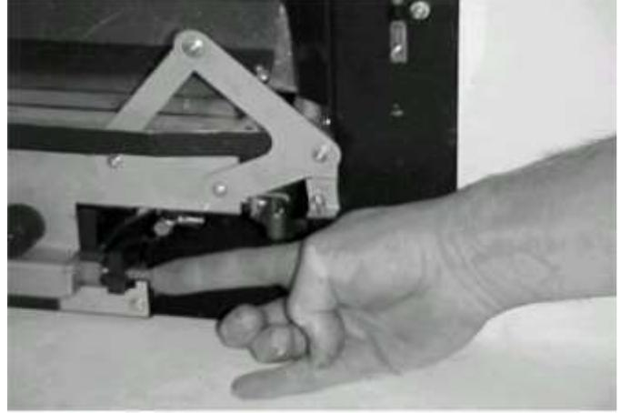
Ensure the spindle is pushed back inside the control valve as far as possible. Ensure the bell crank mechanism is swung up to give easy access to the gas connection point as shown.
