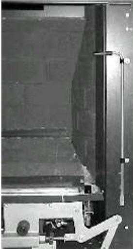
Flip the slide control lever round so that the rubber-capped end is protruding out to the right as shown in the left-hand picture. Check that it slides freely up and down in the nylon slide guides. Remove the nyloc nut with a 7mm A/F spanner as shown.
