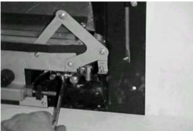
Cut a cross slit in the rubber grommet and feed the appliance onto the 8mm-gas supply pipe. Position the restrictor elbow supplied either as shown or on top of the valve to the left of the inlet elbow using the cutout provided.
